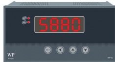
外形尺寸:160×80×125mm 开孔尺寸:152 +1 ×76 +1 mm
